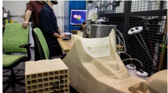
Figure 3: Ford Motor Company is evaluating the Stratasys Infinite Build 3D printer for large-scale 3D manufacturing of automobile components.[44]
